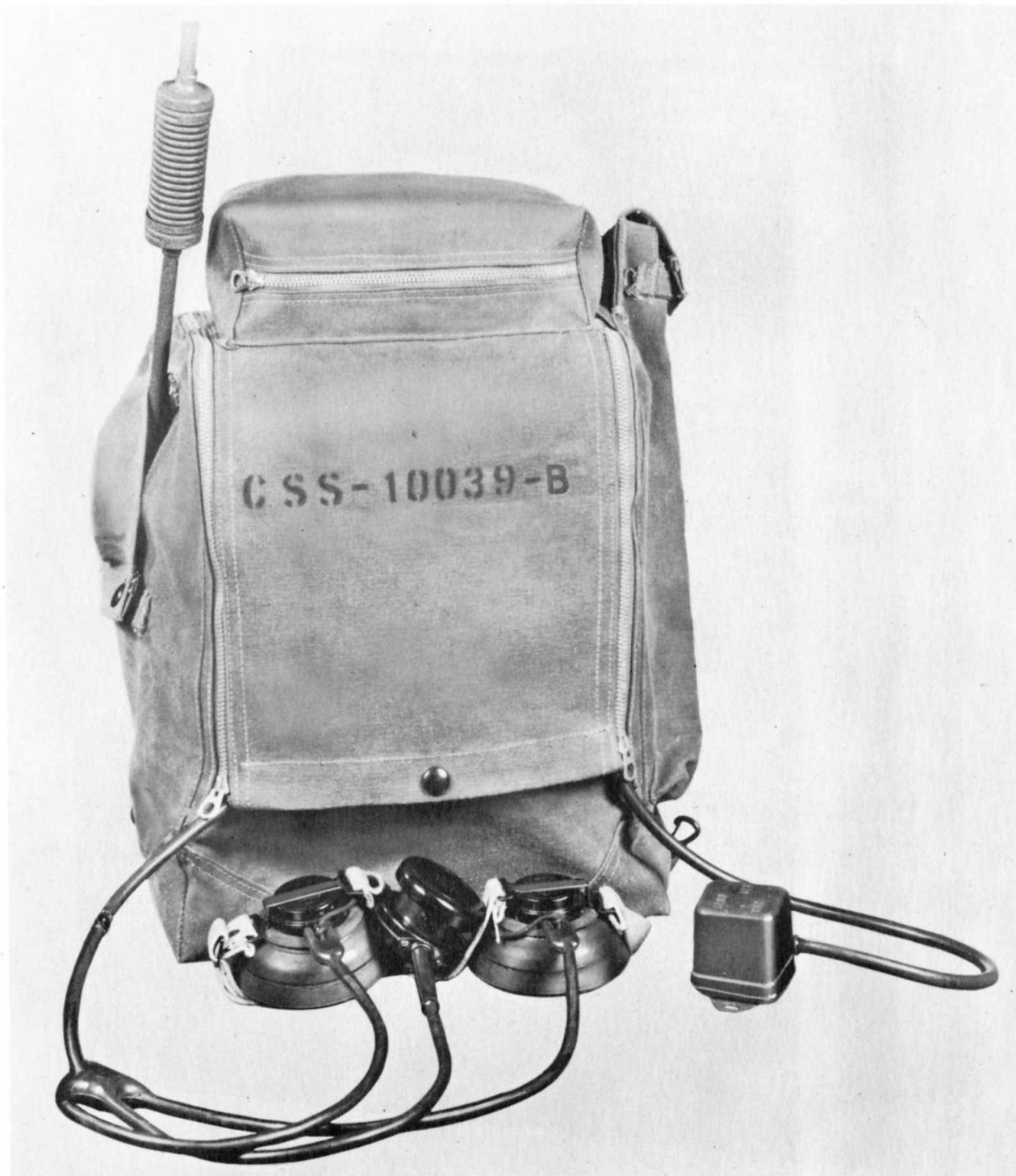
Fig. 8—Navy Model TBY-8 Equipment Assembled for Operation on a Man's Back
